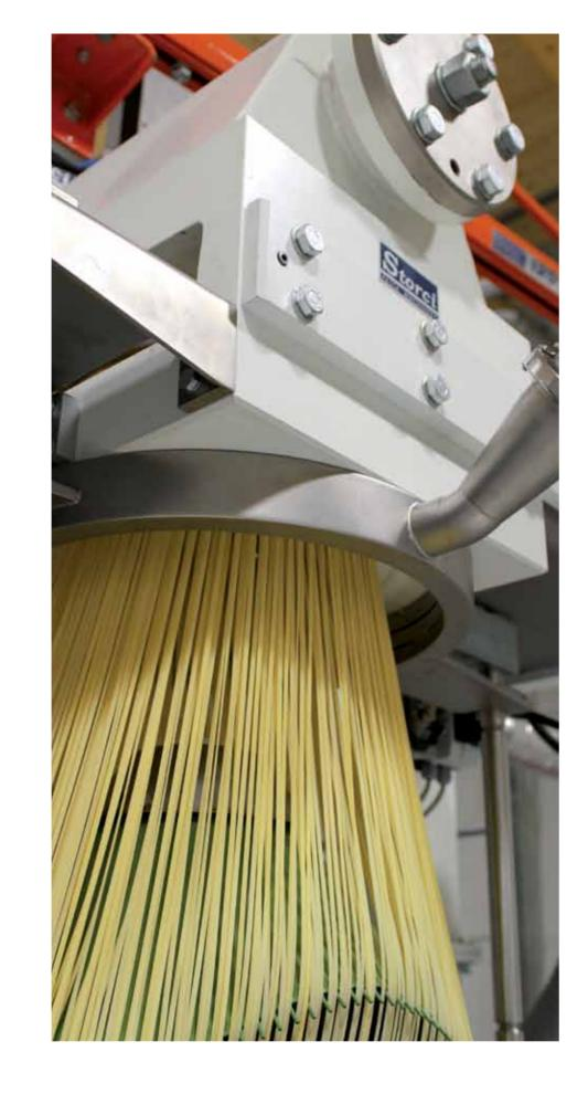
Following the great success of last year with the launch of the Omnia 1000/800, we have created today, thanks to a series of technical and technological adjustments, an extra upgrading of the line, making the new **Omnia** 1200/1000 that can produce up to 1200 kg/h of short pasta and 1000 kg/h of long pasta.
