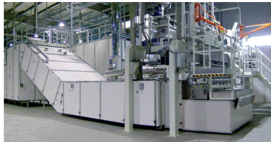
CTA line: continuous pre-drying phase with inclined tier which also serves as an elevator (Fava Storci).
